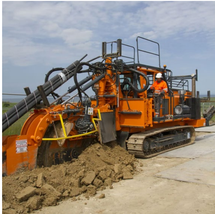
Plate 4-21: Example of cable trenching machine (Source: Equinor)
