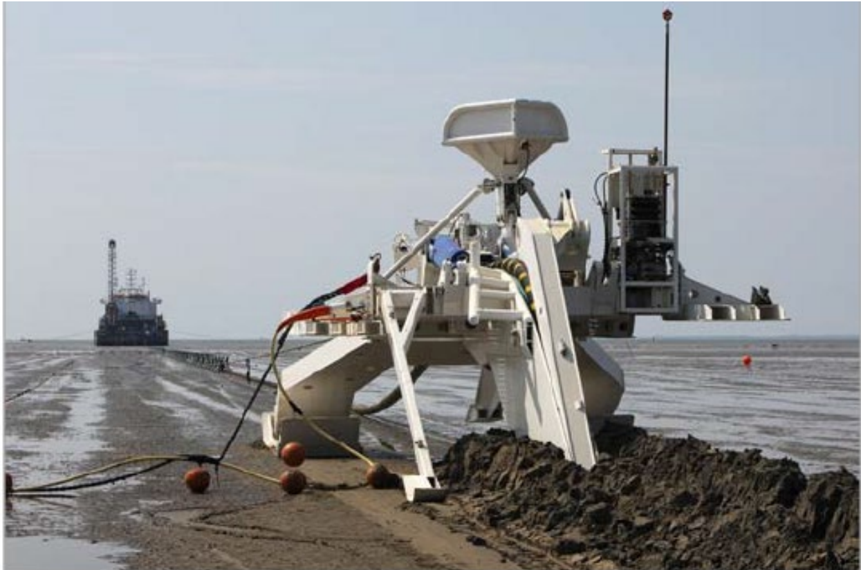
Plate 4-10: Example of a non-displacement plough (Source: Equinor)
